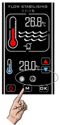
In this mode the controller will heat whenever it is receiving flow during a timed on period and 'Priority of Heating' will take place whenever the timer is 'OFF'.
