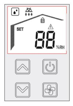
When the dehumidifier is turned on the display will show 88 and then the program version number for ten seconds. This is to allow the relative humidity sensor to sample the air and to take a reading. The display will dim after 90 seconds of no keys being pressed.
