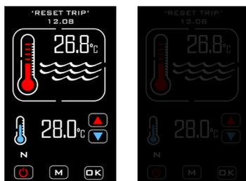
**Remedy:** Remove the black button cover and press red button to reset (see fig. 7) If a positive click is felt, the cause of the tripping **must** be investigated and could be caused by a debris build-up or air pocket trapped inside the flow tube of the heater.
