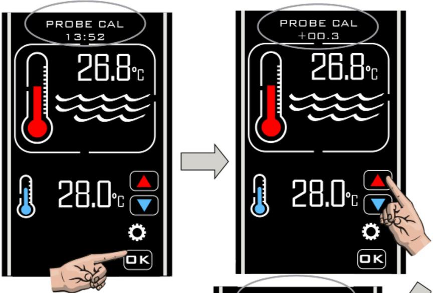
Probe calibration is usually not required. However should you need to make an adjustment take a temperature reading from the pool water with an accurate thermometer then adjust as required.
