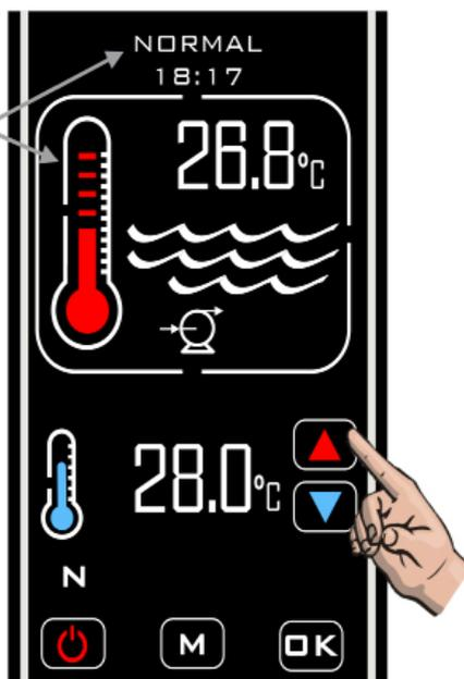
The actual pool water temperature is shown in the upper area of the display. The required temperature is shown in the lower area of the display. The required water temperature can be adjusted by touching the 'UP / DOWN' touch button keys until the required temperature is displayed, adjustments are in 0.1°C increments.
