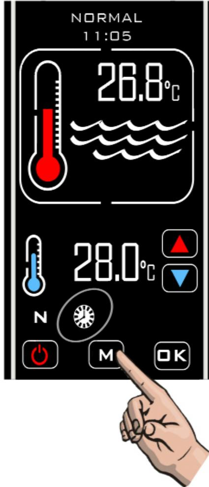
In this mode the controller will only heat during a timed on period and when receiving sufficient flow.
