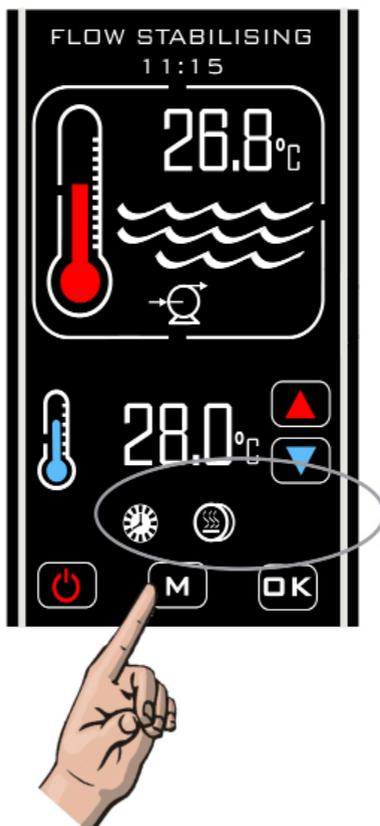
In this mode the controller will heat whenever it is receiving flow during a timed on period and 'Priority of Heating' will take place whenever the timer is 'OFF'.
