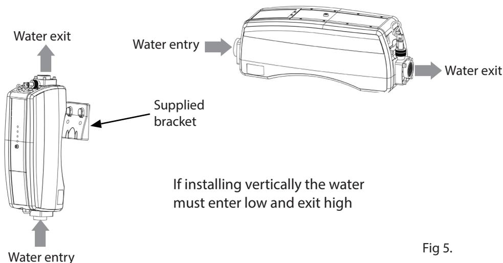
The flow rate of water into the heater must not exceed 17,000 litres per hour (17m<sup>3</sup>/h) / 3,740 UK gallons/hour. A higher flow rate will require the installation of a bypass. The heater will not operate unless the following minimum flow rates are achieved ie:
