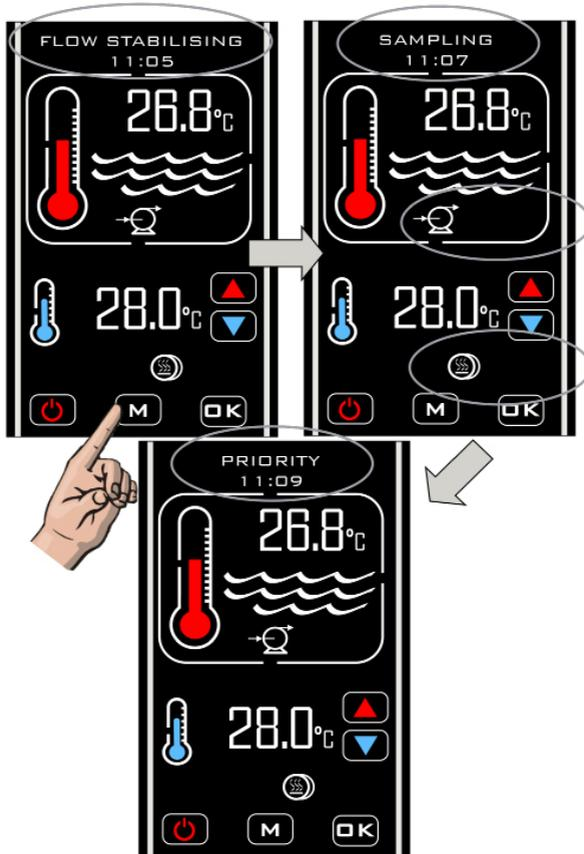
Once the 'Priority of Heating' feature has been enabled the controller will take a water temperature sample every hour and the message 'SAMPLING' will be displayed.
